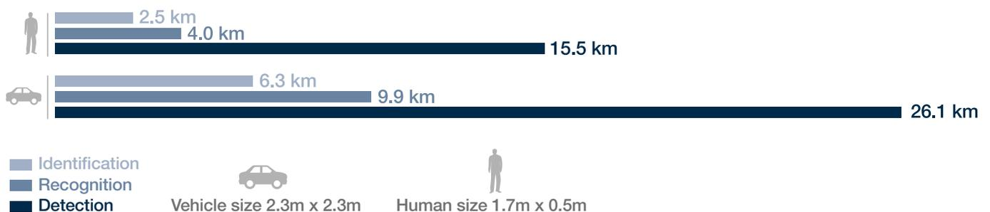
Assumptions: 1280 detector | TRM4 model | Day mode | 0.7 $\mu$ m to 1.7 $\mu$ m spectral range | 25Hz frame rate | Overcast daylight irradiance | 0.2 path radiance factor | 0.2km<sup>-1</sup> atmospheric attenuation coefficient | 50% detection probability | Human and vehicle target 50% reflectivity | 15% background reflectivity
